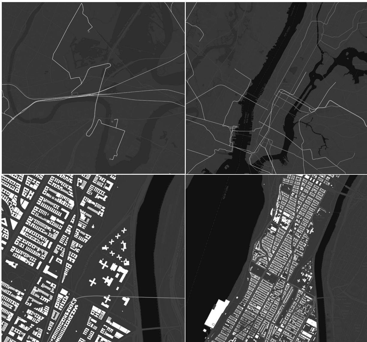
Figure 3. Diagram of underground rail distribution system. Warehousing locations (top left), subway network and nodes into NYC (top right), Polo Grounds HCDC site location (bottom left), on-foot/e-bike distribution network (bottom right).
